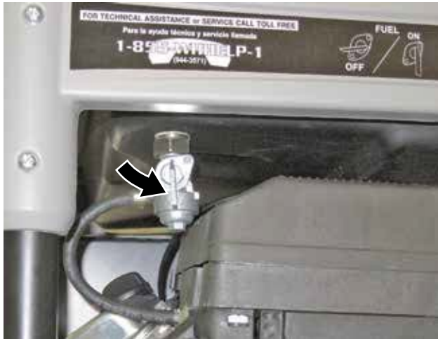
Figure 27 – Fuel Shutoff Valve in the ON Position
