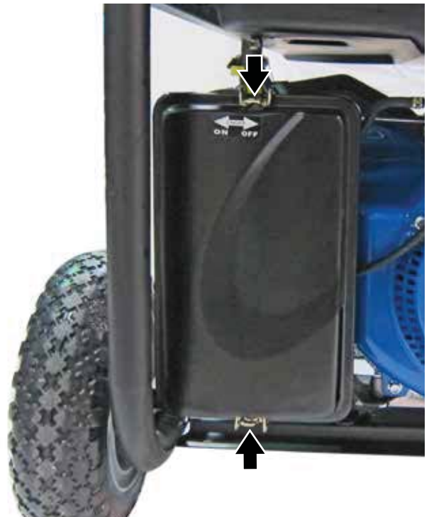
Figure 52 – Installation of Air Filter Cover
