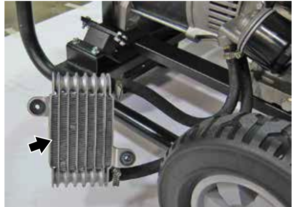
Figure 62 – Oil Cooler Fins
