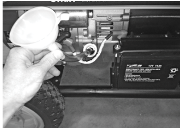
Figure 40 – Adding Engine Oil
