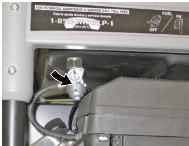
Figure 32 – Fuel Shutoff Valve in the ON Position
