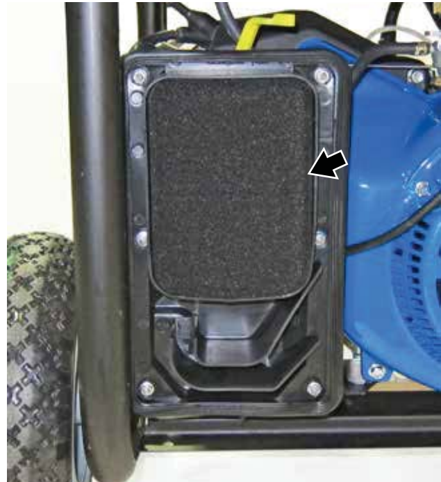
Figure 48 – Removing Coarse Outside Air Filter
