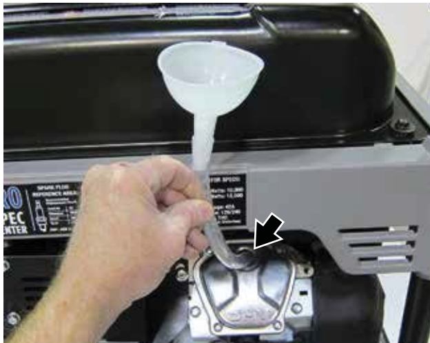
Figure 39 – Adding Engine Oil
